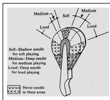
Figure 2. Areas of the hammer to be pierced, depending on the desired amount of voicing (Fletcher and Rossing, 1998, 372).
