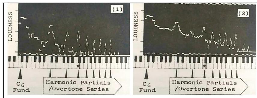
Figure 3. Spectrum analysis of non-percussive attack (1) and percussive attack (2) (Figure adapted from Richerme, 1997).
