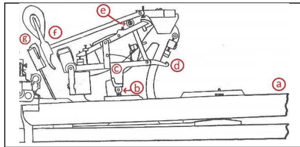
Figure 1. Grand piano action system. Labels have been added to highlight the parts of the mechanism active in the stages described in the text. (a) Key. (b) Capstan. (c) Whippen. (d) Jack. (e) Hammer knuckle. (f) Hammer. (g) Backcheck (Figure adapted from Comparetto, 2017).
